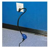
Load Tester plugged in-line with the device
