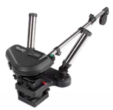
2116 HIGH PERFORMANCE PROPACK The number one choice in performance Downriggers for the charter captain. Equipped with 300 ft. of 180 lb. test stainless steel cable and our stainless steel rocket launcher dual rod holders. 36"-60" 1 1/4" telescopic stainless steel boom.
