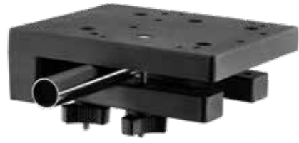
1027 RAIL MOUNT Fits up to 1 1/2" round rails, including oval-shaped wooden rails. Transfers the downward pressure to the boat gunnel. Fits all Scotty Downriggers (except Laketrollers) and can be used with 1026 Swivel Mount. Dimensions: 6 1/8" x 7 7/8"
