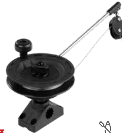
1073 BRACKET MOUNT Mounting bracket permits mounting on a flat deck surface or on the side of a gunnel or transom. The mounting design gives 360° of rotation. Comes with a 241 Side Deck mount. 1 ft. per turn of the spool. Includes 1181 mini power grip line release.
