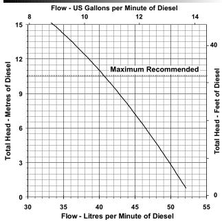
**Current Draw** 12V = 12 Amps @ 3m head 24V = 6 Amps @ 3m head
