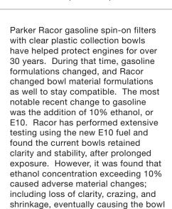
In addition to high ethanol concentrations, other factors such as age, temperature, ultraviolet light, and various fuel additives may negatively impact clear filter bowls.
