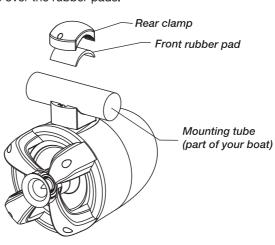
6 - Insert (2) bolts through each rear clamp into the front clamps and tighten each bolt until you feel resistance. Then tighten each of the four bolts a few turns, and repeat until all are fully tightened. By tightening all equally, you will greatly improve the safety of the mounting.
