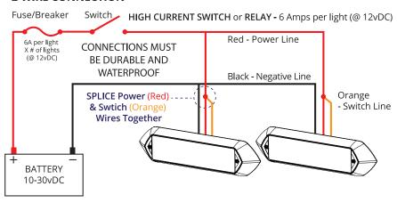
**NOTE:** The JAVELIN can also be wired in a standard two wire installation as well by simply connecting the red and orange wires together and powering via an appropriately rated switched power buss.
