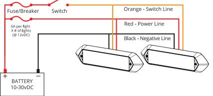
To use the 3-wire system, simply connect the red and black 10-30VDC lines to an appropriately fused power buss with constant power and the Orange wire to a switched +10-30VDC buss referenced to the same ground as the power lines.
