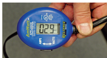
Small electric motor continuous load.
