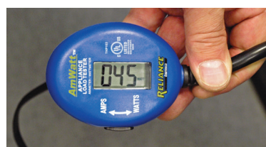
Small electric motor start up load.
