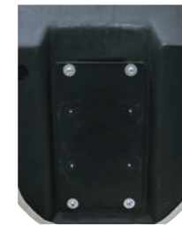
Bucket Seat Underside Shown with 8WD399-1 Mounting Plate
