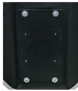
Bucket Seat Underside Shown with 8WD399-1 Mounting Plate
