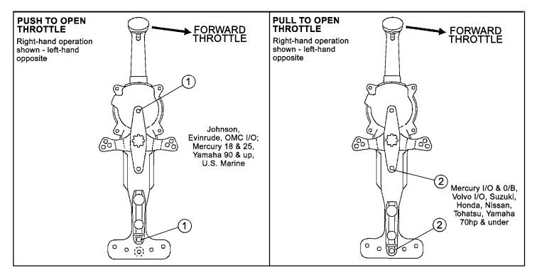
FIGURE 3b CONTROL CABLE CONNECTING POINTS - BY THROTTLE ACTUATION TYPE
