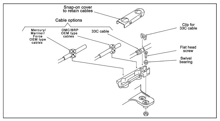
FIGURE 4 - CABLE CONNECTIONS, CONTROL END
