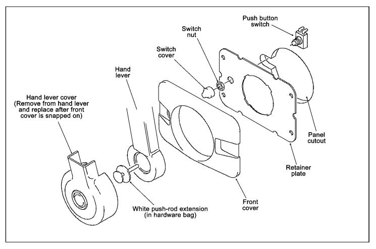
FIGURE 5 - SIDE MOUNT, INSTALLATION
