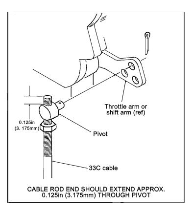
FIGURE 6 - 3300/33C CABLE TERMINAL CONNECTION
