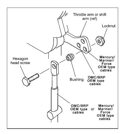
FIGURE 7 - OMC/BRP & MERCURY/MARINER/FORCE OEM TYPE CABLE TERMINAL CONNECTION
