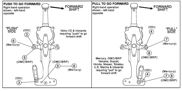
FIGURE 3a CONTROL CABLE CONNECTING POINTS - BY SHIFT ACTUATION TYPE
