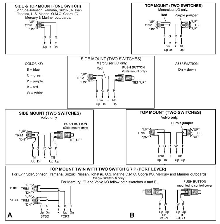
FIGURE 10 - "TRIM" & "TILT" SWITCH CONNECTIONS
