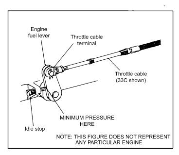
FIGURE 8 - THROTTLE CONNECTION
