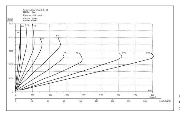
CAPACITY RANGE (based on water at 20°C/68°F)
