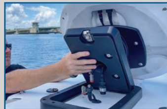
Step 3: Disconnect the cables
