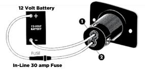
Mounting the receptacle requires a 1 <sup>1</sup>/<sub>8</sub>" hole to be drilled. Select a location where the boats structure will not be weakened. Also, mount on a vertical surface to lessen the amount of water that can enter the receptacle. Alternatively, you may want to mount the receptacle using the Scotty L-bracket (included in your Downrigger kit)
