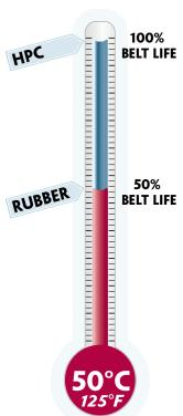
Fenner Drives HPC V-Belts are different in two significant ways. First, they are made of custom reinforced polyurethane elastomers with excellent resistance to high operating temperatures. Second, the unique link design results in belt constructions which limit flex induced heat build-up; a greater surface area also dissipates any heat generated more effectively as compared to a solid construction rubber V-belt... a lower internal belt temperature = a longer belt life.
