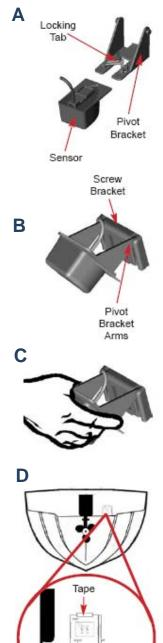
Alignment Arrow 4. The bracket is designed for a standard 13° transom angle. To determine if the plastic shim is needed, position the transducer at the desired location. Using a straight edge, compare the underside of the transducer relative to the underside of the hull. The stern (trailing edge) of the transducer should be 1/16" - 1/8" (1 - 3 mm) below the bow (leading edge) of the sensor.
