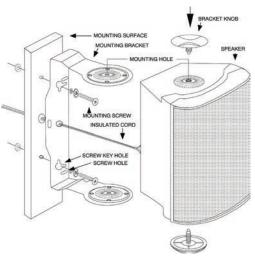
Do not mount the bracket to nonreinforced plaster sheetrock gypsum board). Once the bracket is secure, reattach the speaker using the thumb screws included.
