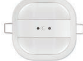
01529.1 IR presence detector, 360° motion range, for ON/OFF lighting, 1-1000 Lux adjustable brightness range, KNX standard, for ceiling installation. Dimensions: 91x91x45 mm
