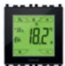
02952 Touch screen thermostat for ambient temperature control of 2 independent zones, KNX standard, NO 4 A 24 V~ relay output + 1 temperature sensor input + 1 programmable digital input - 2 modules. To be installed with dedicated 16723 mounting frame. Depth: 38,5 mm
