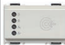
16927.B Transponder card reader for installation outside rooms, KNX standard, 2 NO 4 A 24 V~ relay outputs, 2 inputs, power supply 12-24 V~ 50/60 Hz and 12-24 Vdc (SELV) - 3 modules. Supplied without transponder card. Depth: 36,5 mm
