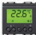
16915 Thermostat for ambient temperature control of 2 independent zones (heating and air-condition- ing), KNX standard, NO 4 A 24 V~ relay output + 1 temperature sensor input + 1 programmable input - 2 modules. Depth: 36,5 mm
