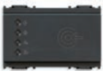
16927 Transponder card reader for installation outside rooms, KNX standard, 2 NO 4 A 24 V~ relay outputs, 2 inputs, power supply 12-24 V~ 50/60 Hz and 12-24 Vdc (SELV) - 3 modules. Supplied without transponder card. Depth: 36,5 mm
