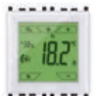
02952.B Touch screen thermostat for ambient temperature control of 2 independent zones, KNX standard, NO 4 A 24 V~ relay output + 1 temperature sensor input + 1 programmable digital input - 2 modules. To be installed with dedicated 16723.B mounting frame. Depth: 38,5 mm
