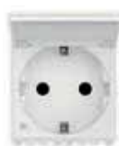
20208.C.B SICURY 2P+E 16 A, German, with cover - 2 modules. Depth: 31,2 mm
