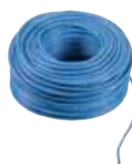
732H/100 Due Fili Plus cable for internal laying, 2x1 mm 2 twisted conductors, PVC sheath, operating temperature -25/+70 °C, insulation degree 450/750 V, not suitable for running through underground channels - 100 m bundle
