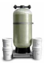
Parker Village Marine Remineralizer Systems offer pH neutralization of RO water and are specifically engineered to operate with Village Marine PW and SW Series Watermakers. The media restores a buffer capacity to raise pH and reduce fresh water "aggressiveness" against metal pipes and fixtures.
