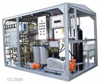
The Sea Water Series reverse osmosis desalination systems are designed to provide potable water in demanding environments. Its rugged, efficient design allows high through-put of water with minimum electric power use. The Sea Water Series systems are quiet because the mounting of the motors and Aqua Pro pumps isolates and minimizes vibration transfer to the vessel's hull or the RO system enclosure.
