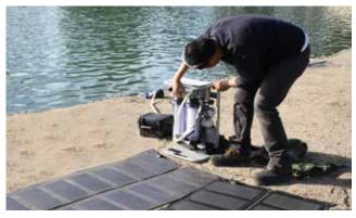
Parker Village Marine RUF units provide fresh water filtration that is truly portable and independent. The RUF-25 or RUF-30 will process 25 or 30 gallons per hour from 12 volt vehicle auxiliary power (cigarette lighter). Optional lightweight folding solar power version provides 25 gallon per hour production from sunlight. Water treatment includes 20 micron sediment filtration, carbon filtration, ultrafiltration membranes and ultraviolet radiation.
