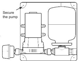
Fig 2 - Recommended Kit Mounting Orientation
