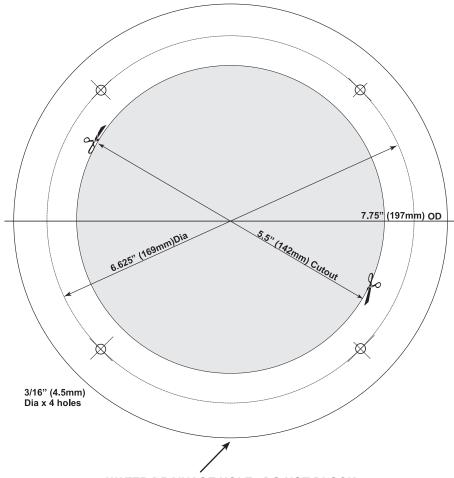
WATER DRAINAGE HOLE - DO NOT BLOCK
