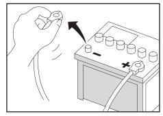
To avoid potential shorts in the electrical system, be sure to disconnect the (–) battery cable before installation. Use this unit with a 12-volt battery and negative grounding only.
