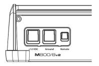
The M800/8v2's "+12 VDC" and "Ground" connections are designed to accept 4 AWG power wire. 4 AWG is the required wire size for this amplifier.
