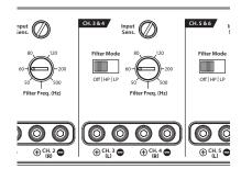
1) "Filter Mode" Control: The M800/8v2 employs a 12dB per octave filter for each pair of channels. Each of these filters can be configured independently into one of two filter types or defeated completely by way of the three-position "Filter Mode" switches:
