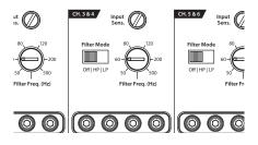
To properly set the amplifier for maximum clean output, please refer to Appendix A (page 14) in this manual. After using this procedure, you can then adjust any or all "Input Sens." levels downward if this is required to achieve the desired system balance.
