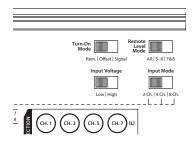
The "Low" position on the "Input Voltage" switch selects an input sensitivity range between 200mV and 2V for all input channels. This means that the "Input Sens." rotary control for each channel section will operate within that voltage window. If you are using a source unit with conventional preamp-level outputs, this is most likely the position that you will use
