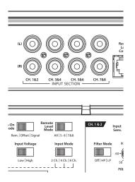
If you wish to send eight discrete channels into the M800/8v2, simply use all eight inputs and set the "Input Mode" switch in the "8 Ch." position.
