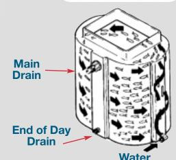
The molded-in slosh guard keeps slosh and wet decks to a minimum. The light dome in the bottom of the tank eases nighttime access and prevents fish from hitting the walls in the dark. All tanks come with "L" mounting brackets, a durable molded cover (ModelPF-42 has a solid poly cover) and are covered by a no-nonsense 1 year warranty.
