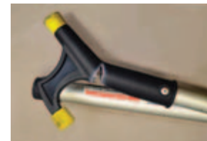
West Marine® snapped at 550 lbs. (249 kg).
