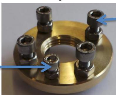
Locking ring showing nuts and bolts assembled
