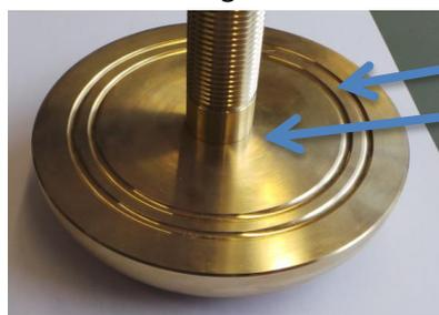
Apply Sealant around these grooves and around the stem
