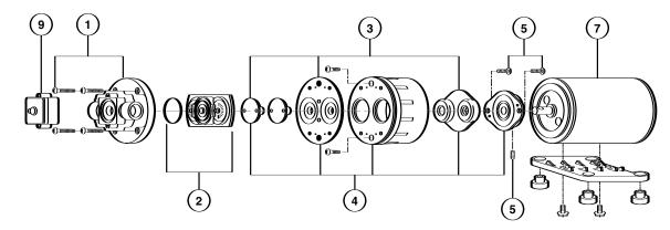
Quite often when a pump is worn or defective the one failed component has overburdened others. To avoid frequent aggravating repairs, Flojet offers service kit assemblies making repairs as quick and easy as possible.
