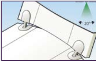
Intelli-Hinge permits hinging concave surfaces
