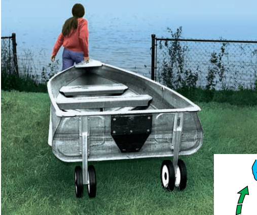
Removal of the two lower lockpins allows the wheels to be pivoted and locked in an upright position while underway. Removal of all four pins releases the entire wheel assembly.
