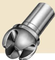
All AFTCO butts can be special ordered with a "ball gimbal." Precision machined from 6061-T6 aluminum, AFTCO ball gimbals make it more comfortable when planting a rod butt in your stomach while stand-up fishing without a fighting belt. A round design helps prevent deck scarring, and extra heavy, tapered feet make for a snug fit to gimbal pins. To special order, write "BG" after the Catalog Number.
