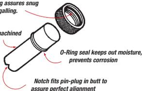
O-Ring seal keeps out moisture, prevents corrosion
